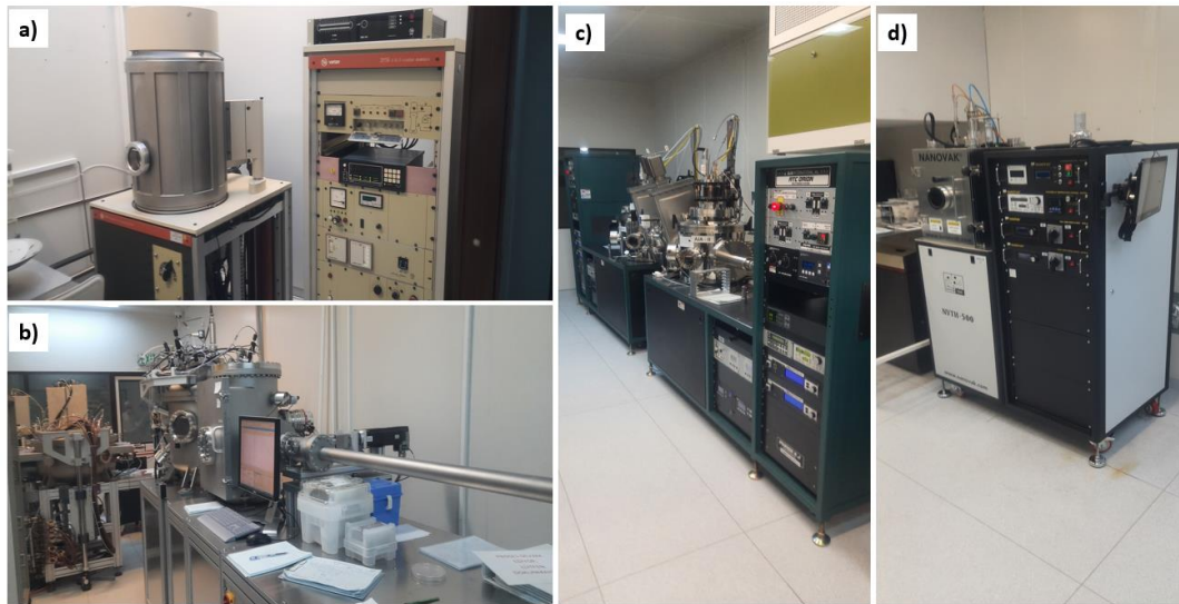
Figure 3.6 a) Varian 3119 Thermal Evaporator System, b) BESTEC Sputtering System, c) AJA Sputtering System, and d) Nanovak NVTH 500 Thermal Evaporator System
