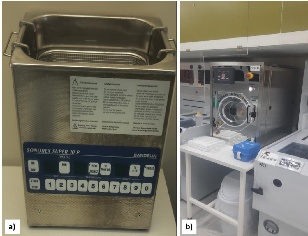
Figure 3.10 a) Ultrasonic Cleaner for Lift-Off Process and b) Avenger Ultra-Pure 8 SRD System
